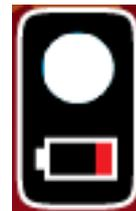
**Low Battery Indicator:** Lights when the battery requires replacement.
