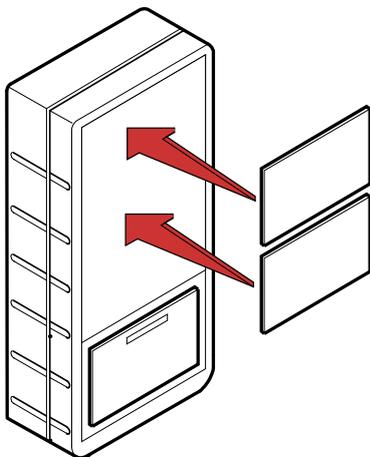
**1.** If required you can attach the self-adhesive magnetic strips to the rear of the Key Fob tester.
