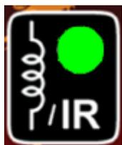
4. If a signal is received then the Infra-Red LED will illuminate for the duration of the transmission. This may be continuous or just short bursts, depending on the key fob.
