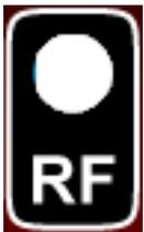
**RF Indicator:** Lights RED when an RF signal of 433MHz is received. Lights Green when an RF signal of 868MHz is received.
