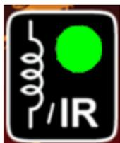
4. If a signal is received then the IR/Transponder LED will illuminate for the duration of the transmission. This may be a continuous burst or just short bursts depending on the vehicle.
