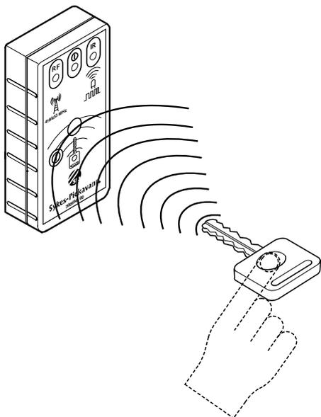
3. Point the key fob at the tester Infra-Red receiver window and operate the button.
