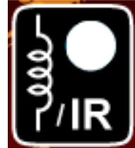
**IR/Transponder Coil Indicator:** Lights when an Infra-Red signal or 125KHz transponder coil signal is received.
