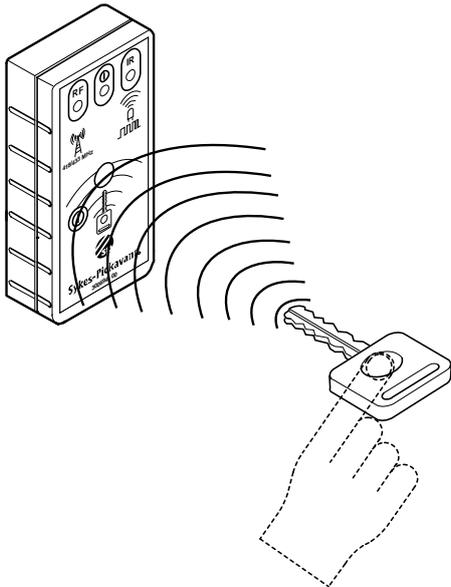
3. Point the key fob at the tester and operate the button.
