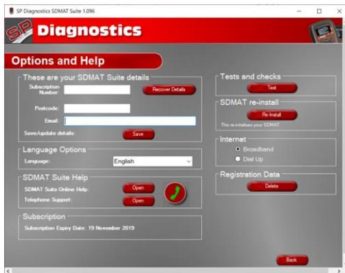
4. Selecting the **'Tests and checks'** button allows you to perform tests to verify that your SD-MAT is functioning correctly and that you are able to connect to the website and download the latest software.
