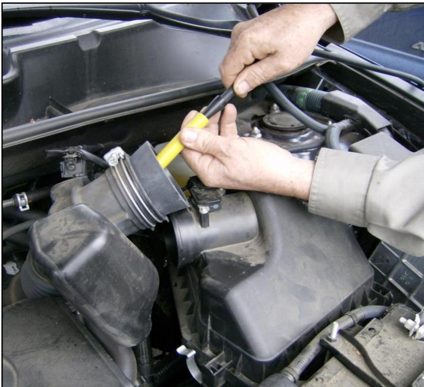
Use cone to access intake system and connect smoke supply hose to cone.
